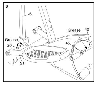
Attach the Left Pedal Arm (21) to the left Upper Body Arm (6) with an M8 x 25mm Patch Screw (70), an M8 Washer (64), and a Pedal Leg Cover (23).
